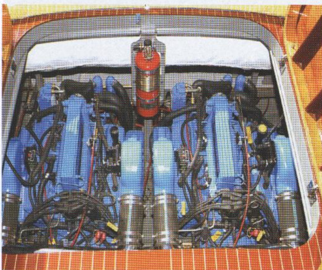
The Piranha's Twin 5.7 Liter Crusader V-8s
