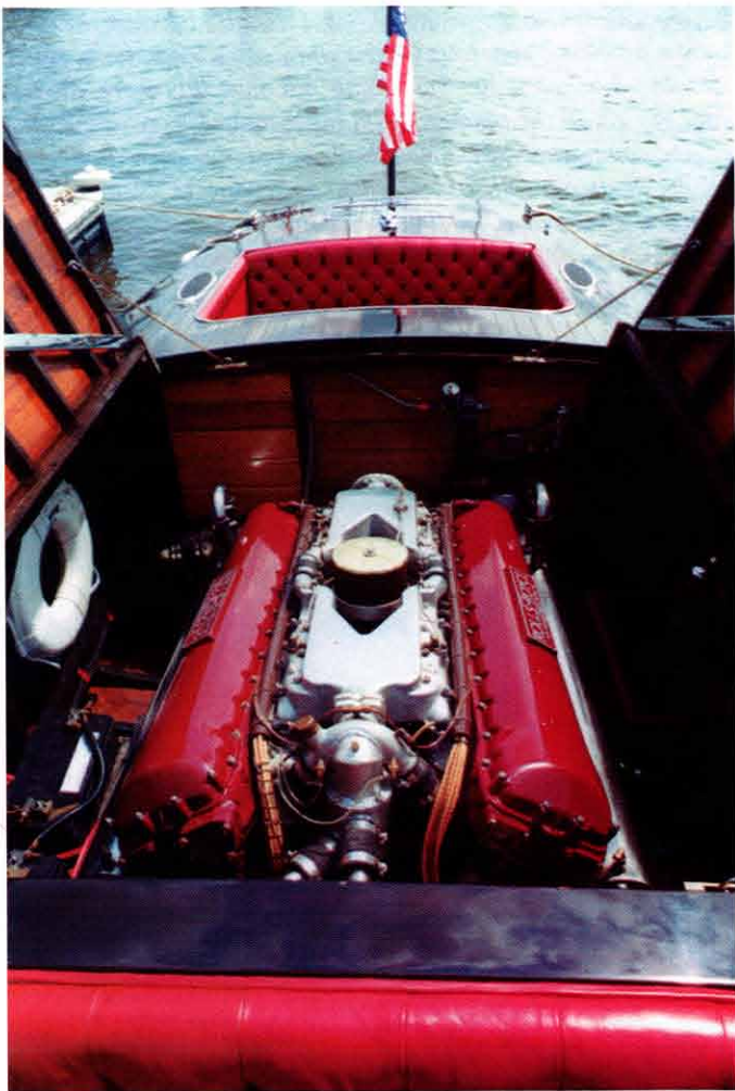
Rolls Royce 'Meteor' – 1650 Cubic Inch – 628 hp.
